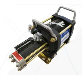
Haskel Gas Boosters consist of a large area reciprocating air drive piston directly coupled by a connecting rod to a small area gas piston. The gas piston operates in a high pressure gas barrel section. Each gas barrel end cap contains high-pressure inlet and outlet check valves. The air drive section continuous reciprocating action when air is supplied to the air drive inlet.
